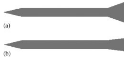
Figure 1. Geometry of the axi-symmetric projectile: (a) r/D=1.25 and (b) r/D=0.75 .
